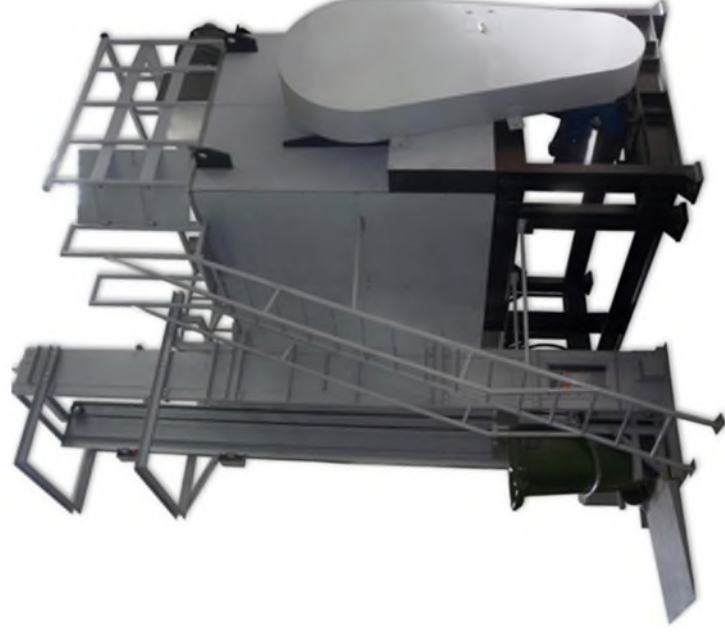
Weimar Composting Machine (1000kg capacity)
