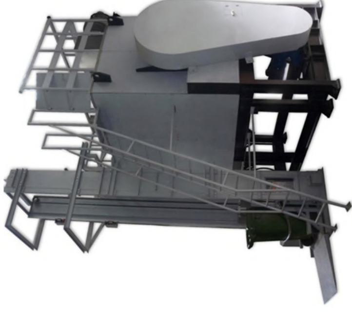
Weimar Composting Machine (500 kg /day capacity)
